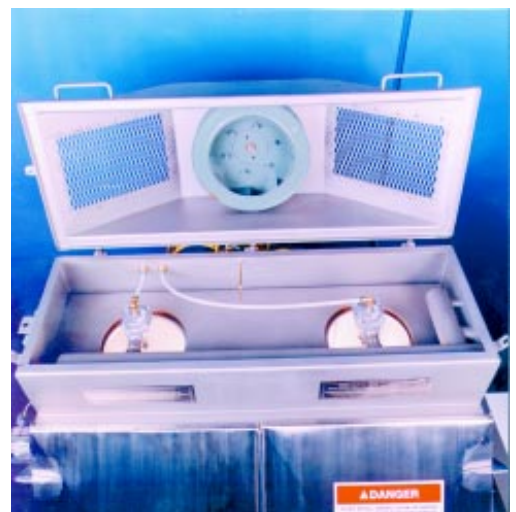
Internally mounted fan, pulse jet cartridge cleaning divertors and compressed air manifold.
