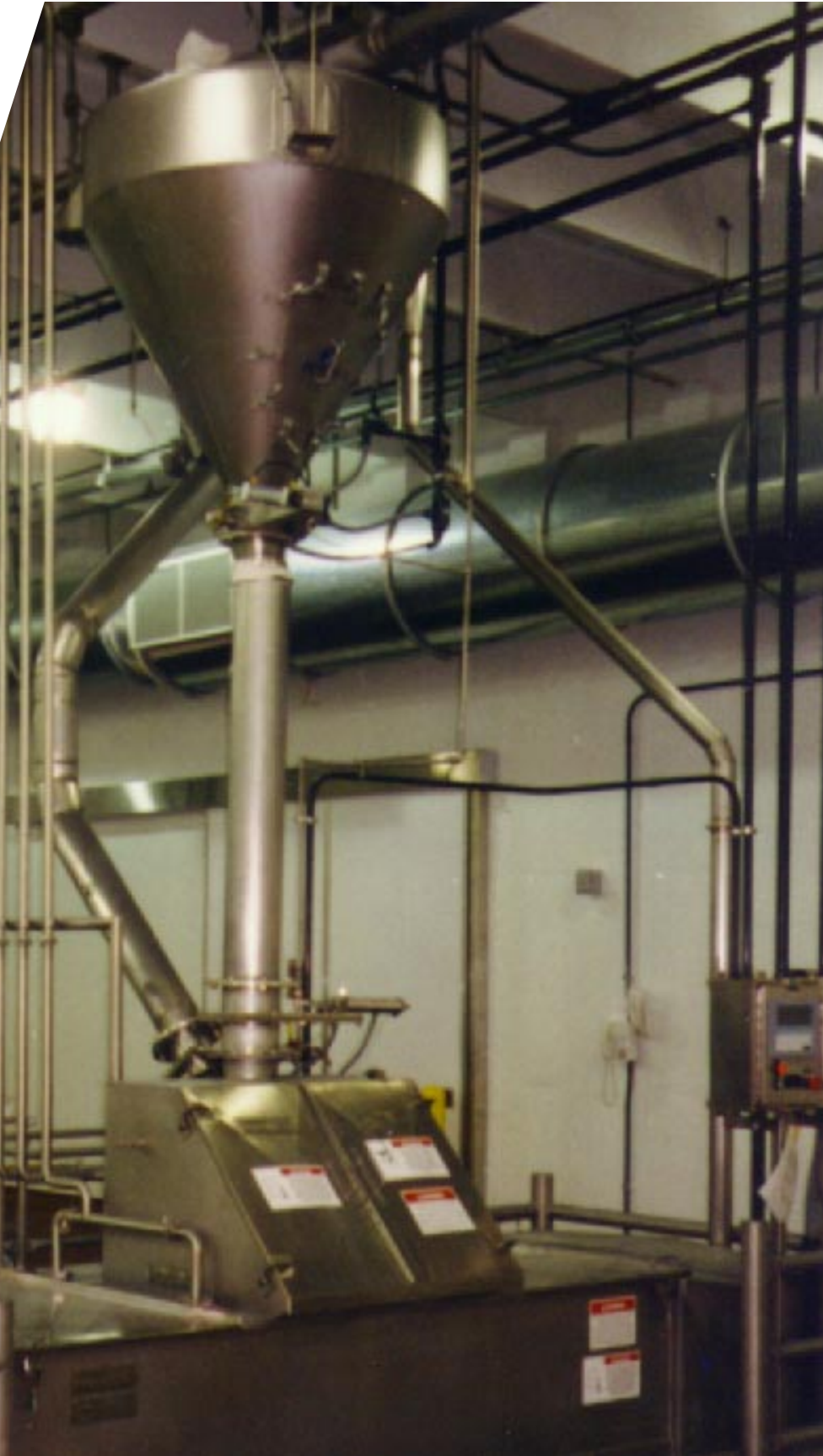
hop workstation, double ribbon blender, batch weighing hopper and remote dust control system.
