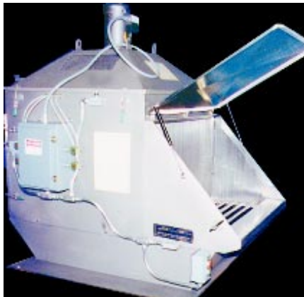
Four cartridge, flange mounted bag dump work station to act also as a bin vent while blowing into mixer
