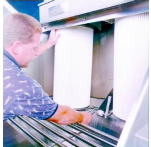
Easy to remove filter cartridges capture dust particles as small as submicron size and returning all airborne product to the hopper.
