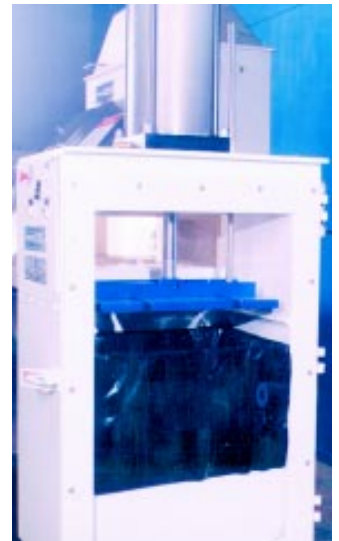
PBC-50 Pneumatic Bag Compactor (door removed to show interior)
