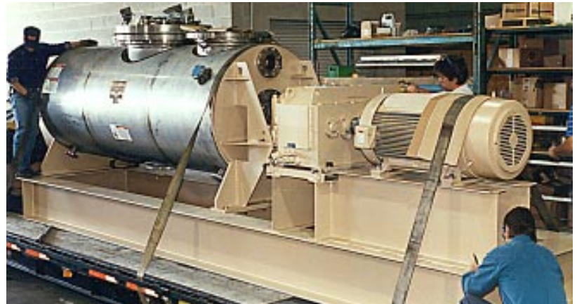
CPB-135 designed as a vacuum dryer/reactor for "dutching" cocoa - delivered as a complete system with jacketed dust collector and vacuum pump.
