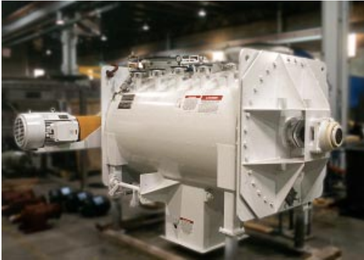
CPB-45 for corrosive rubber reclamation application. Mixer is Kynar® coated carbon steel with Hastelloy components.
