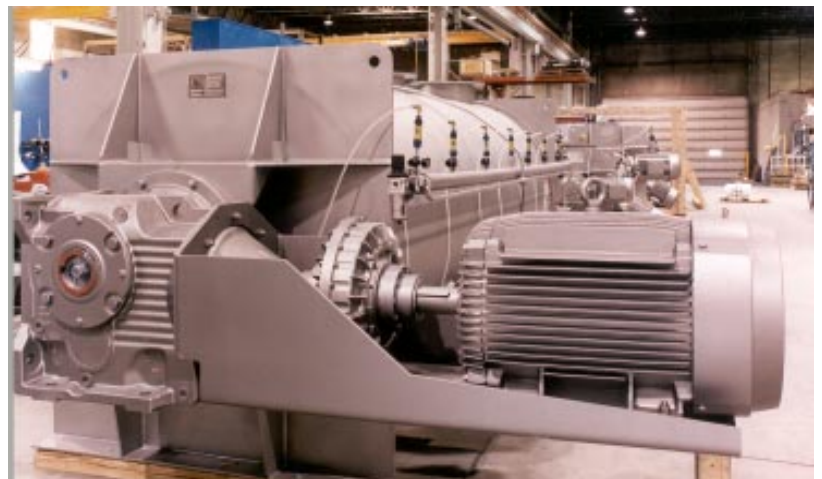
CPB-175 with shaft mounted gear box, scoop mounted motor, and fluid coupling, plus compressed air header for shaft seals.
