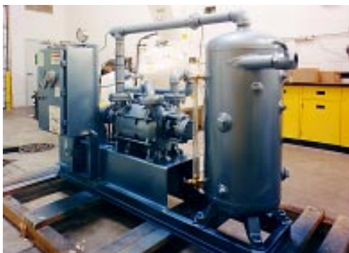
Our fully equipped test lab includes ancillary equipment such as this vacuum pump for reacting and vacuum drying
