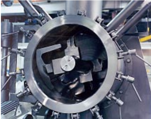
APS maintains an inventory of mixers, dryers, and reactors with switchable tools (paddles/plows) for testing at our test lab (below), or in-plant testing. (Shown T 4.5 with Paddles)
