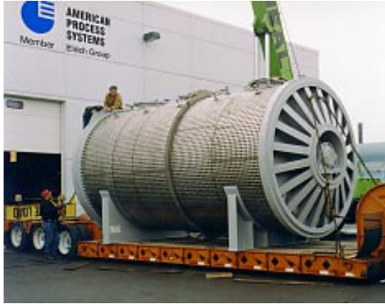
CPB-1200 Cylindrical Reactor rated 150 psi internal pressure, Alloy 20, ASME heat jacketed
